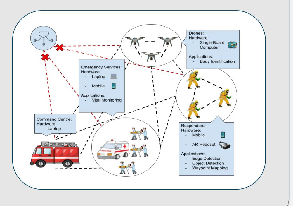
propose a mesh network of devices where each device can offload a portion of its workload to nearby peers. In such a scenario, each application can be considered critical. Thus we aim to explore a novel mechanism to enhance computational offloading that can adaptively adjust resources provisioned to each offloaded task when the network is under strain.
