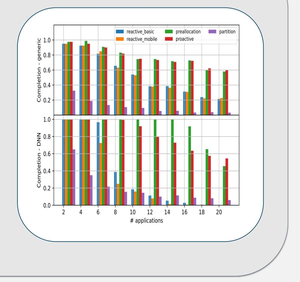
We conducted experiments with each type of offloading algorithm where we offloaded N (1 -> 20) applications, conducting each experiment 20 times.
