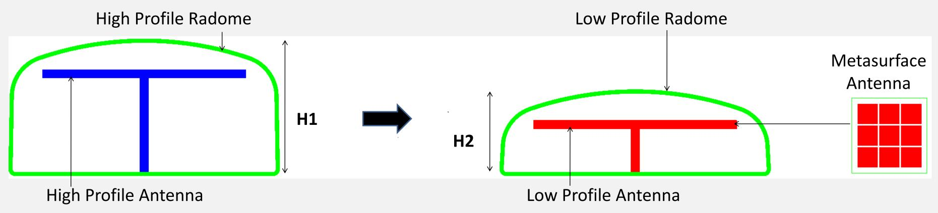
2) Frequency Selective Surface/ Metamaterial technique to be used in interleaved Multiband antenna to provide cloaking for different frequencies in different antennas.
